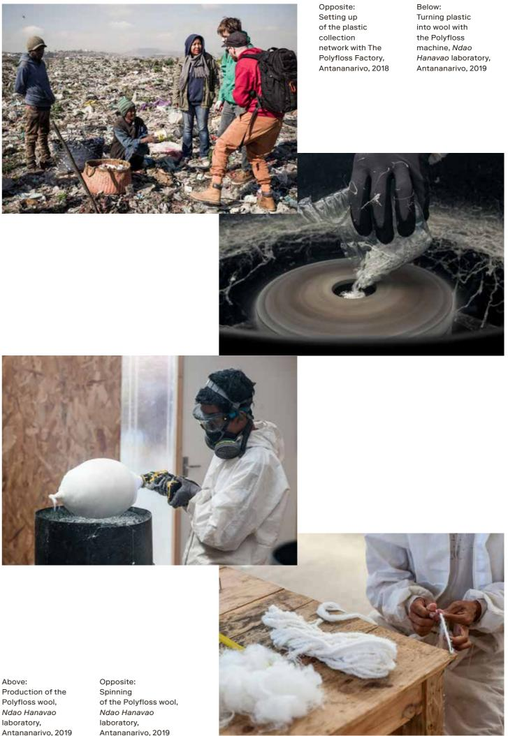
Plastic waste collected from the waste dumps of Antananarivo and sorted by a network of collectors then enters the production phase in the workshop set up by the two guest designers and young trainees, where the recycled plastic is transformed into finished products such as design pieces and staple items. The plastic is also sold in the form of panels, wool, rolls of felt, etc. as a building material and as a raw material for local crafts.
