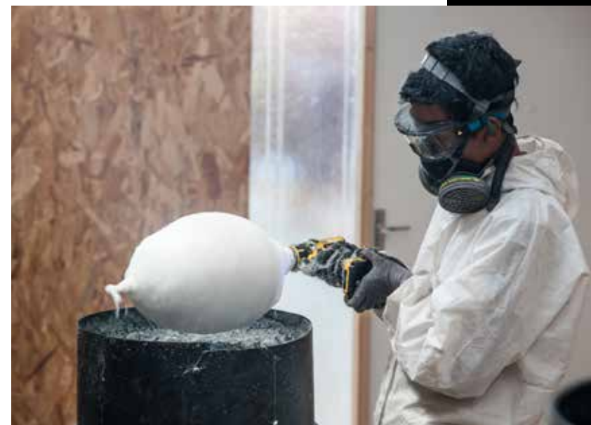
Above: Production of the Polyfloss wool, Ndao Hanavao laboratory, Antananarivo, 2019
