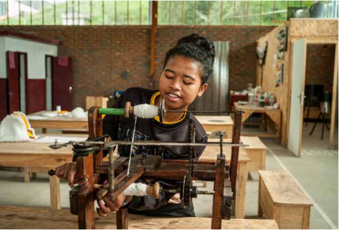
Spinning of the Polyfloss wool with a spinning wheel, Ndao Hanavao laboratory, Antananarivo, 2019
